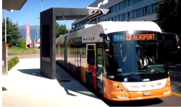
Figure 1: A TOSA bus charging at a bus stop.
